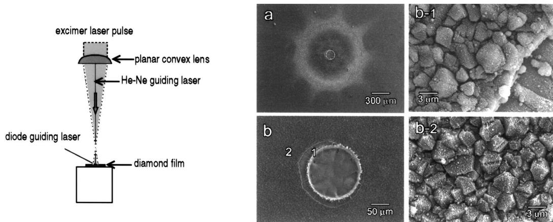
Fig. 1. Experimental setup and SEM micrographs for the excimer laser irradiation in atmospheric condition: (a) the irradiated spot and surroundings; (b) the irradiated spot; (b1) magnified view of area 1 from (b); and (b2) magnified view of area 2 from (b).
