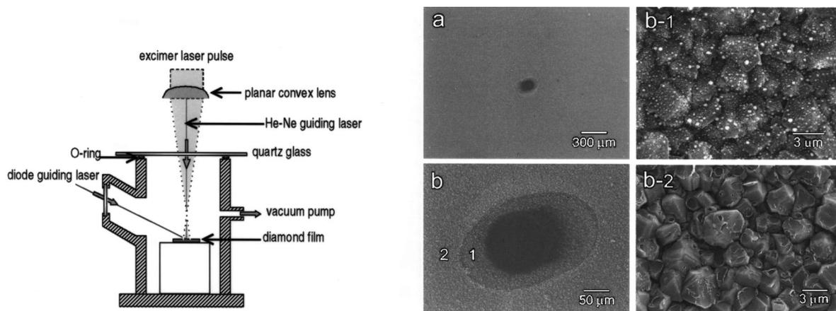
Fig. 2. Experimental setup and SEM micrographs for the excimer laser irradiation in vacuum condition: (a) the irradiated spot and surroundings; (b) the irradiated spot; (b1) magnified view of area 1 from (b); and (b2) magnified view of area 2 from (b).
