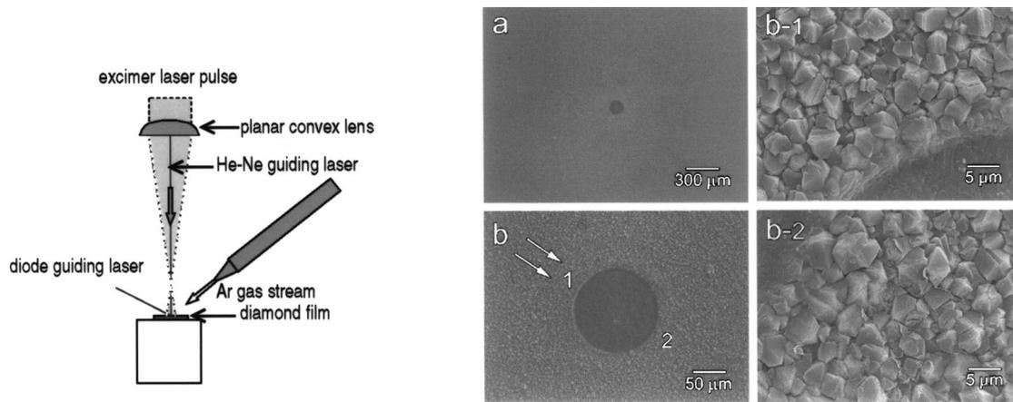
Fig. 3. Experimental setup and SEM micrographs for the excimer laser irradiation in gas-stream condition: (a) the irradiated spot and surroundings; (b) the irradiated spot; (b1) magnified view of area 1 from (b); and (b2) magnified view of area 2 from (b).
