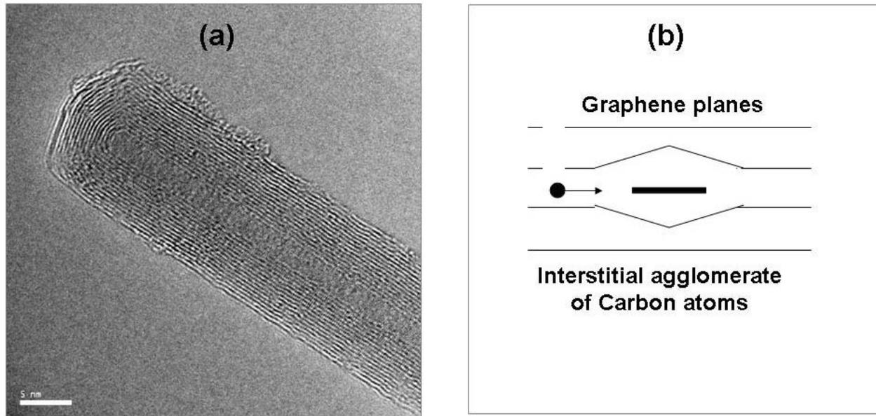
Figure 7. (a) HRTEM image of multi-walled carbon nanotube after 900 sec 86-Krypton irradiation. No displacement damage of the type shown in (b), was observed (Figure 7(b) after Reference 16).
