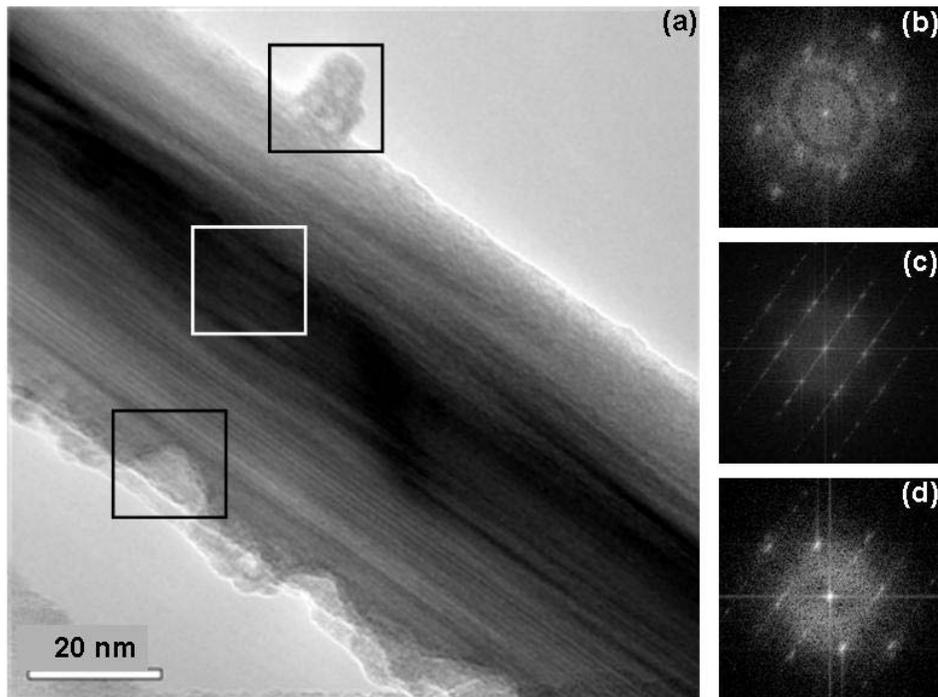
Figure 4. (a) GaN nanowire after 355 Gray 78-Krypton irradiation with corresponding FFTs. (b) Plumbe were shown to be amorphous by strong concentric rings in FFT pattern. (c) The highly crystalline wurtzite core showed no indication of damage. (d) Gouges on lower side did not show strong concentric rings and may have been present in the pre-irradiation GaN nanowire.
