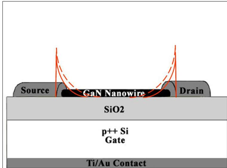
Figure 1. Cross section of GaN nanowire FET. A 150 nm oxide layer is grown on a highly doped p-type silicon wafer functions as the gate. Ti/Au source and drain leads are patterned via electron beam lithography on top of the nanowire, and the Ti/Au gate contact is evaporated on the backside of the wafer forming the global gate. The action of the gate bias  $V_{GS}$  is to raise/lower, and thin/thicken the Schottky barrier at the nanowire/nanotube-metal contact.
