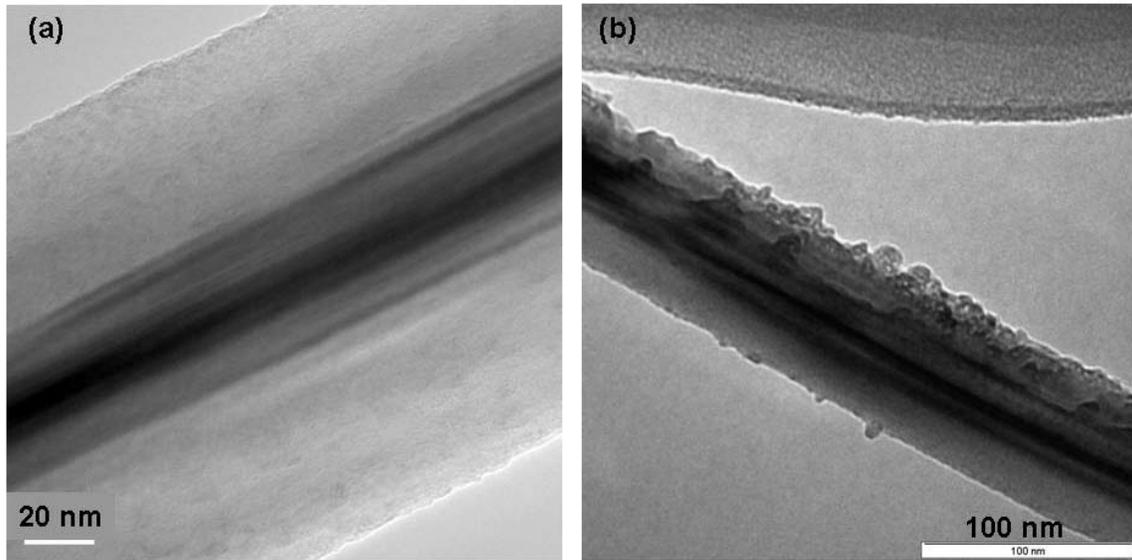
Figure 3. Pre Irradiation GaN nanowires. (a) Most GaN nanowires were highly crystalline with a wurtzite core and coaxial zinc-blende outer layer however (b) defective GaN nanowires were also observed.
