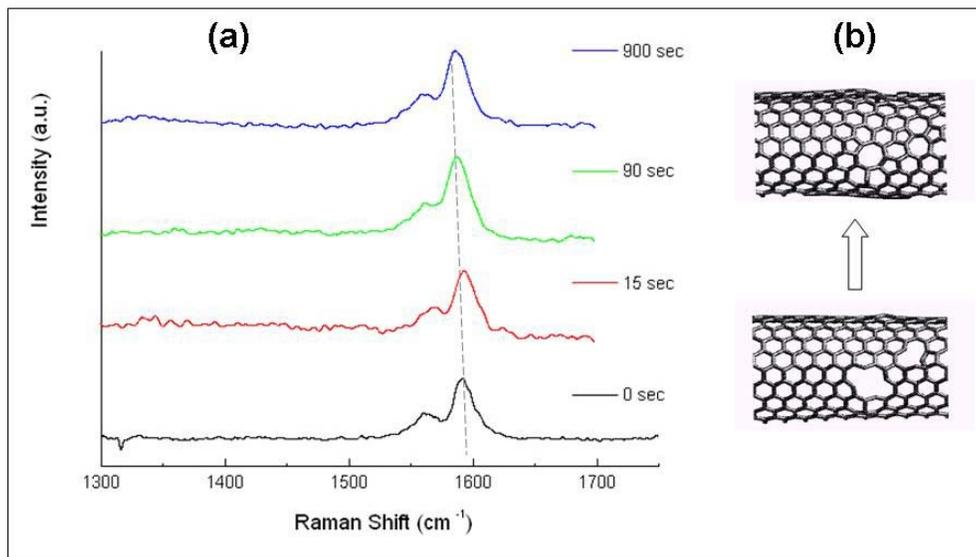
Figure 6. (a) Micro Raman spectroscopy of the tangential modes indicated that the carbon nanotube cylinder was intact for all doses. A slight shift may be due to compressive stress caused by self-healing of displacement damage, as shown in (b) (Figure 6(b) after Reference15).
