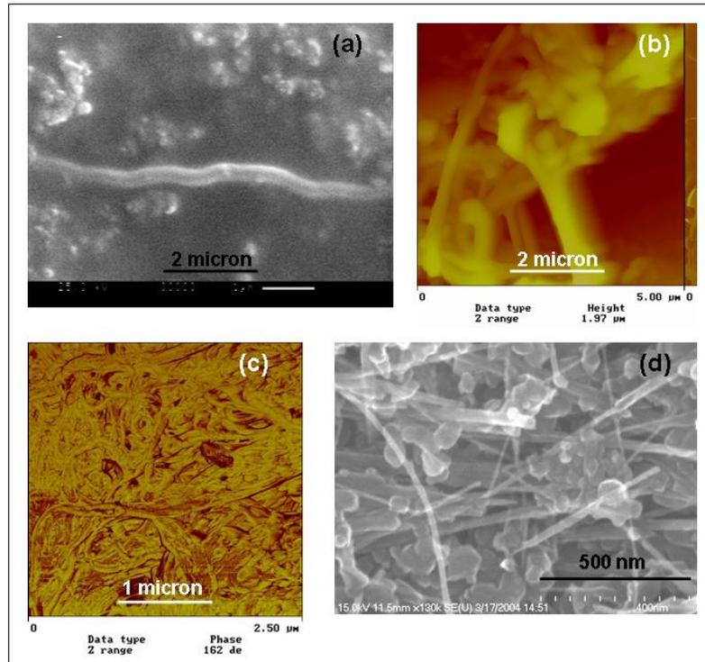
Figure 5. (a) FE SEM of vapor grown carbon fibers, and (b) AFM of electrospun carbon nanofibers indicated substantial structural damage after 900 sec 86-Krypton irradiation. (c) AFM of single walled carbon nanotubes and (d) FE SEM of multi walled carbon nanotubes did not show any obvious structural damage.
