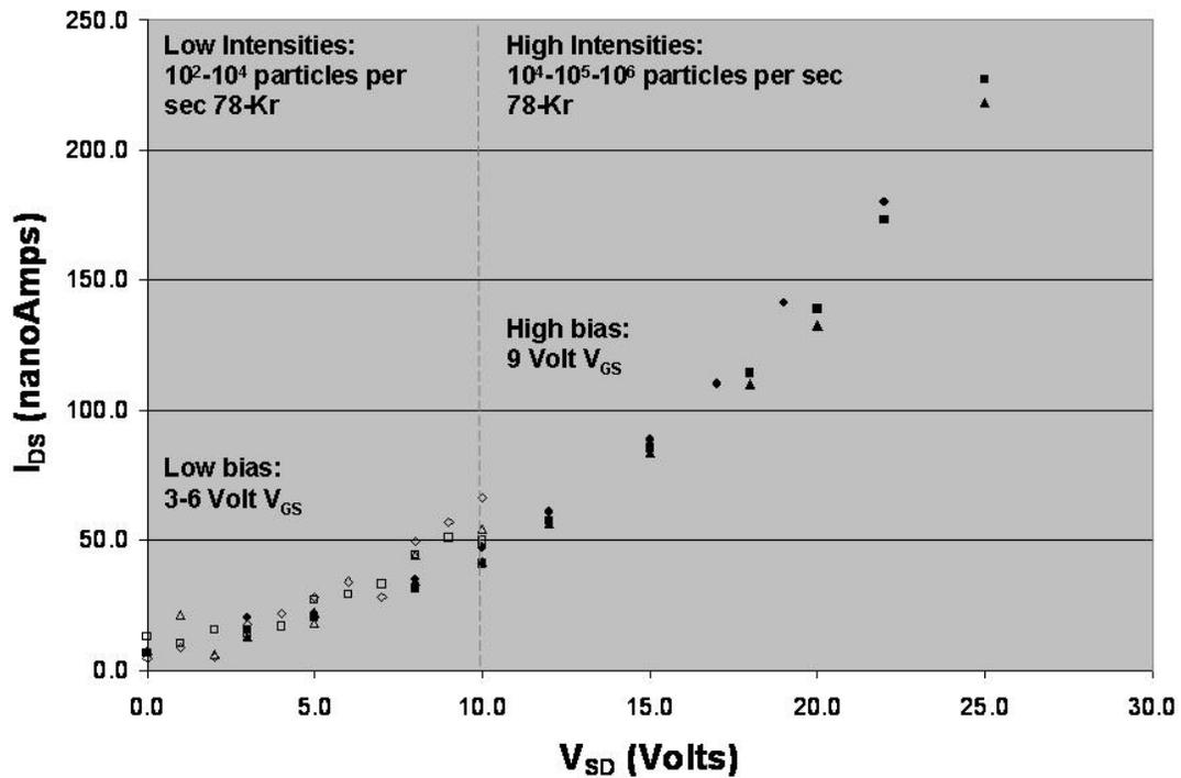
Figure 2. I-V characteristics of actively running GaN NW FET during 78-Kr irradiation.
