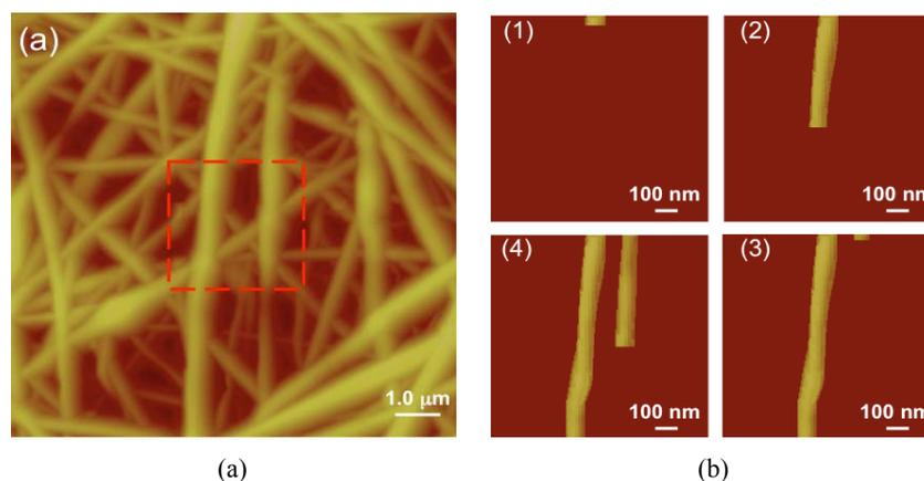
In conventional atomic force microscopy, shown in Figure 1(a), a raster scan with a fixed step-size is employed throughout the image. In SPRM, shown in Figure 1(b), a user-defined coarse-step scan is initiated within user-defined boundaries [red box,
