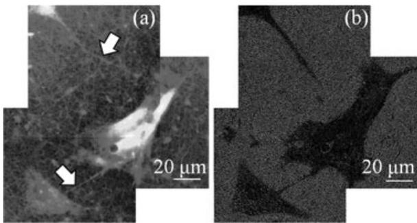
Fig 6. In the composite AFM height image (a), cellular processes and cell edges are indistinguishable from the nanofibrillar background. (b) In the GHPF result, the cellular edges and processes are clearly distinguished from nanofibrillar scaffold.
