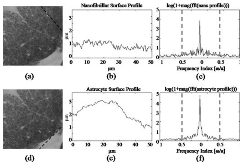
Fig 2. (a) Section measurement of nanofibrillar surface along dashed line, (b) corresponding surface profile, and (c) DFT of nanofibrillar surface profile. (d) Section measurement of cell surface along dashed line (e) corresponding surface profile, and (f) DFT of cell surface profile.
