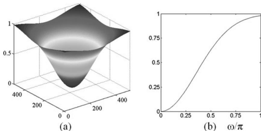
Fig 4. (a) Perspective plot and (b) radial cross section of the GHPF transfer function of order 1 and normalized cutoff frequency 0.5. The zero frequency sample is at the center in (a).
