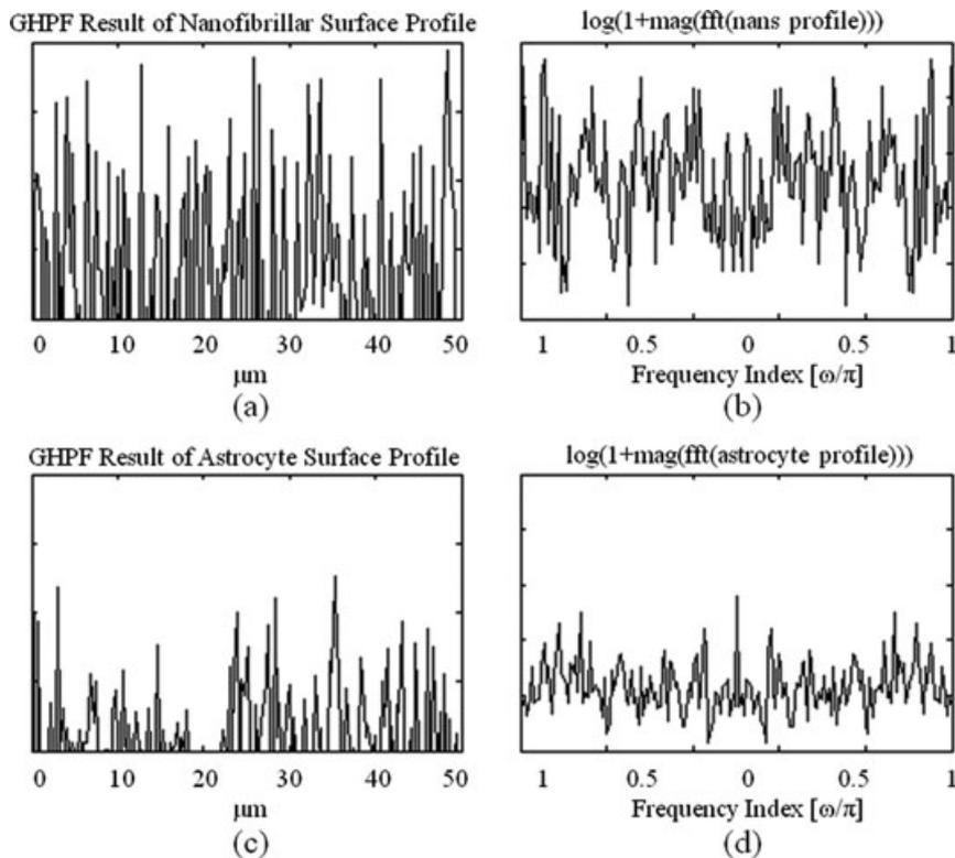
Fig 3. GHPF results (a) filtered nanofibrillar surface profile, (b) DFT spectrum of the nanofibrillar surface profile, (c) filtered astrocyte surface profile, and (d) DFT spectrum of the astrocyte surface profile.
