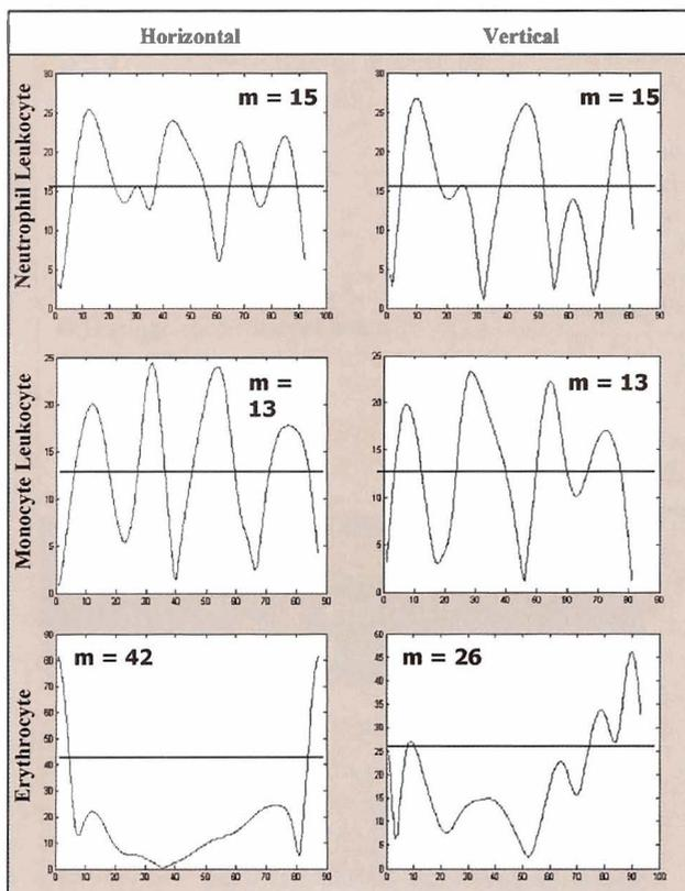
Fig. 3. Continuous wavelet transforms  $W(\sigma, \tau_1, \tau_2)$  shown for horizontal ( $y = 0$ ) and vertical ( $x = 0$ ) axes. The mean value  $m$  is displayed for each plot. Number of zero crossing  $n =$  number of times, the plot intersects the mean line. For all specimens studied, the number of zero crossings  $n < 4$  corresponded to a red blood cell and  $n > 4$  to a white blood cell.
